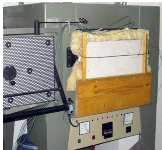
Fig. 8. Concrete panel positioned as a replacement for the furnace door and exposed to a thermal gradient.
