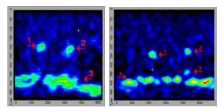
Fig. 10. Tomograms of a concrete block with internal artificial defects, obtained after testing with 36 element antenna array
