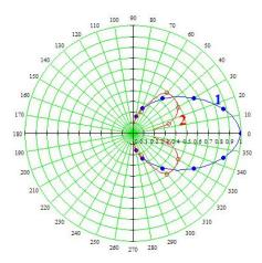
Fig. 17. Directivity pattern of longitudinal and shear waves for a single high-frequency SAT of antenna array with a liquid contact
