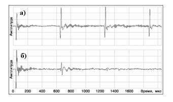
Fig. 12. Echo-signal oscillograms received on anchor bolt end: (a) free lying bolt; (b) built-in concrete bolt
