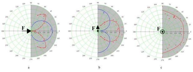
Fig. 8. Directivity patterns of transducers with DPC: a – with normal vibration of the wear tip; b – with tangential vibration of the type, section along the vibration vector; c – with tangential vibration of the type, section perpendicular to oscillation vector; 1 – longitudinal waves; 2 – shear waves
