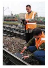
Fig. 14. Rails testing process with the guided wave flaw detector AKR 1224
