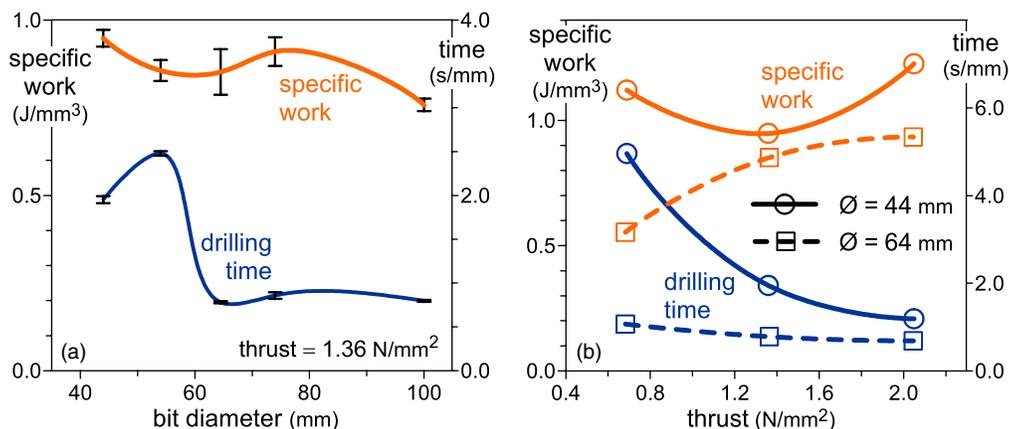
**Fig. 2.** Results of the preliminary core-drilling tests under varying bit diameter and exerted thrust (rotational speed 600 rpm)
