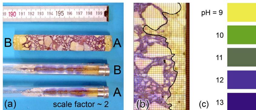
**Fig. 9.** (a) Carbonation depth in a 100-mm concrete cube, determined on a microcore and on two sorted powder samples; (b) local irregularities of the carbonation front; (c) color scale of the pH indicator
