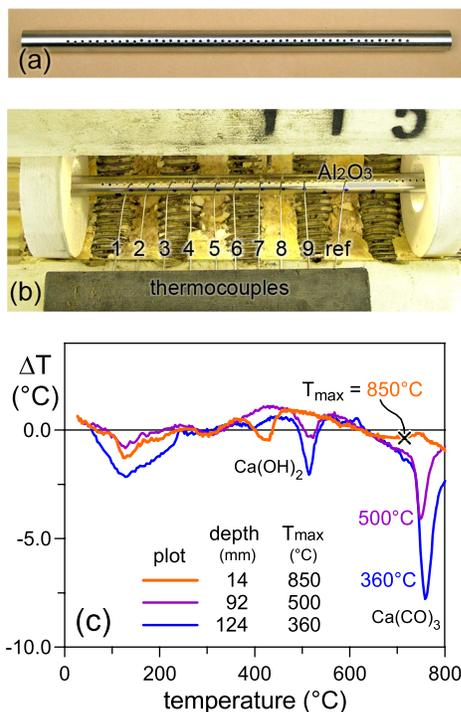
**Fig. 12.** (a) Nickel-chromium perforated pipe to be filled with a sorted sample of drilling-powder; (b) test setup in the split-tube furnace; (c) temperature differentials pertaining to different depths in a heated panel (see Fig. 6)
