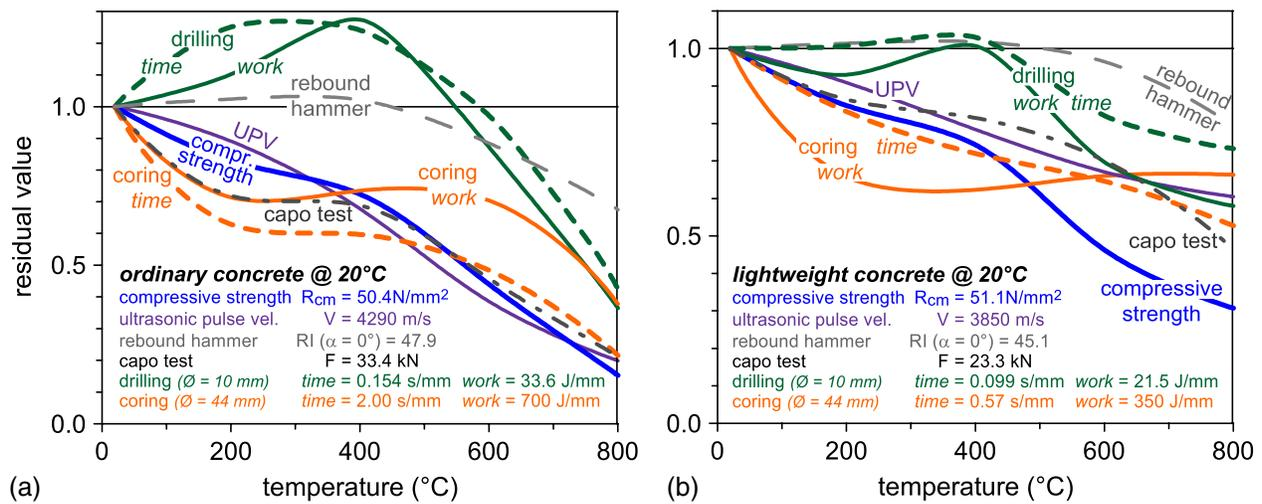
**Fig. 3.** Sensitivity to a uniform thermal damage of some common NDTs and of the core- and hammer-drilling techniques applied to (a) normal and (b) lightweight concrete
