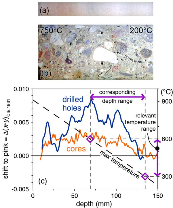
**Fig. 11.** Discoloration of a powder sample and a core taken from the same heated panel and corresponding color variation profiles obtained by means of the digital image analysis
