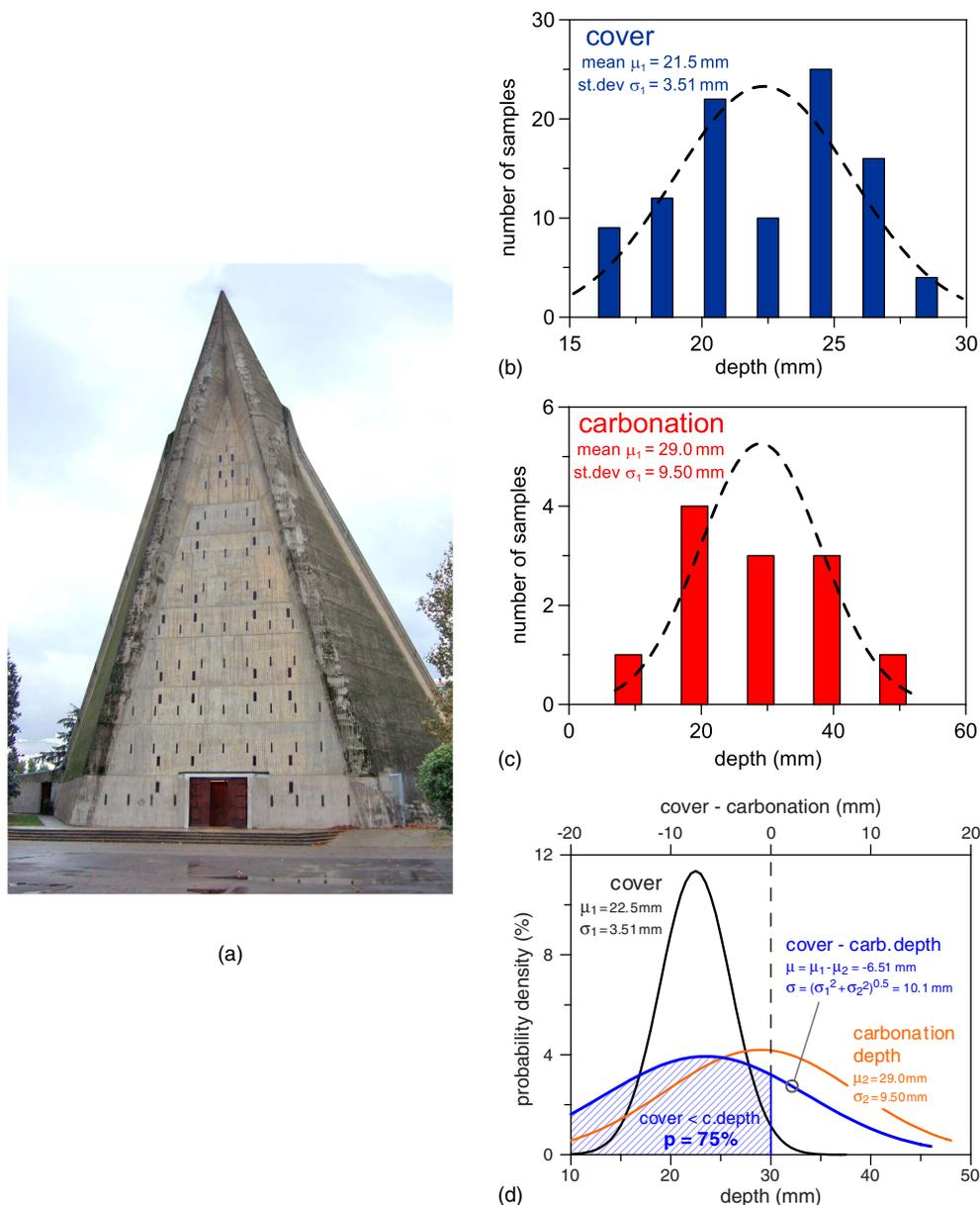
**Fig. 10.** (a) The S. Giovanni Bono church in Milan; comparison among the frequency distributions of (b) the concrete cover, (c) the carbonation depth, and (d) their difference
