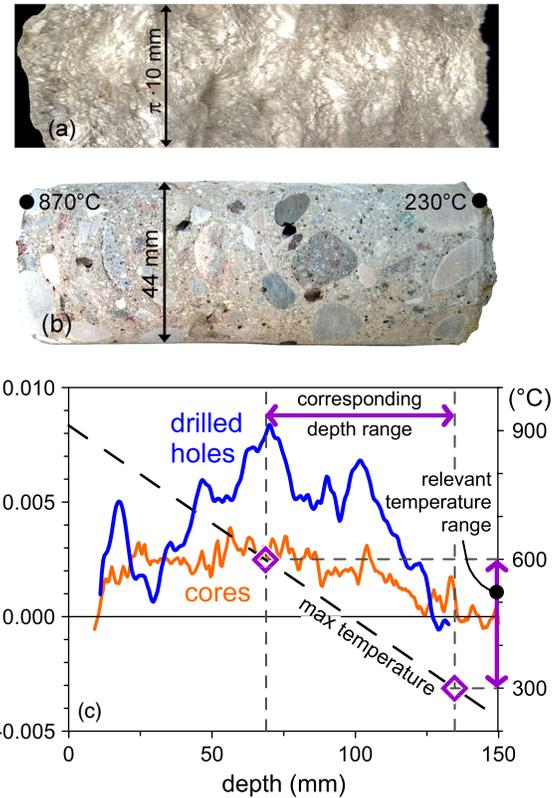
**Fig. 6.** View of (a) the unwrapped inner surface of a drilled hole and (b) a core taken from the same concrete panel submitted to a thermal gradient; (c) color alteration profiles within the panel determined by means of the digital image analysis
