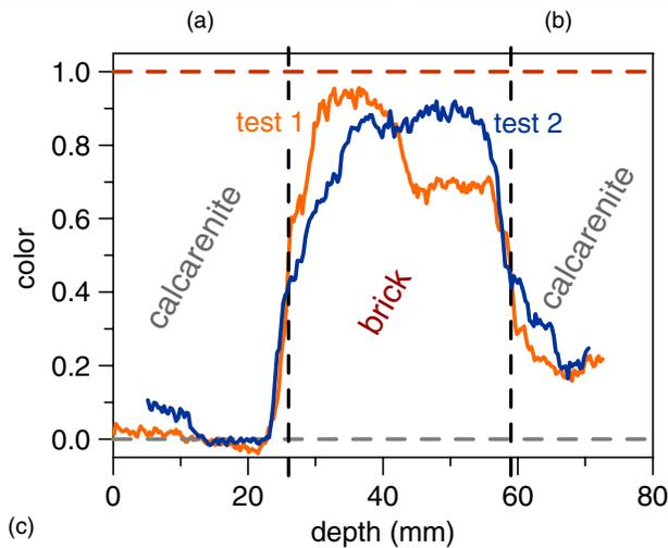
**Fig. 8.** (a) Layered specimens of alternate colors; (b) powder sample extracted from the central calcarenrite-brick specimen; (c) diagrams of the color variations along the powder sample (the abscissa is scaled to the actual depth in the drilled hole)
