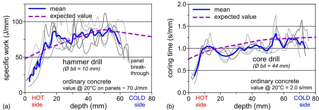
**Fig. 4.** Profiles of the most responsive (a) drilling and (b) coring resistance indicators for a concrete panel that has been exposed to a steep thermal gradient
