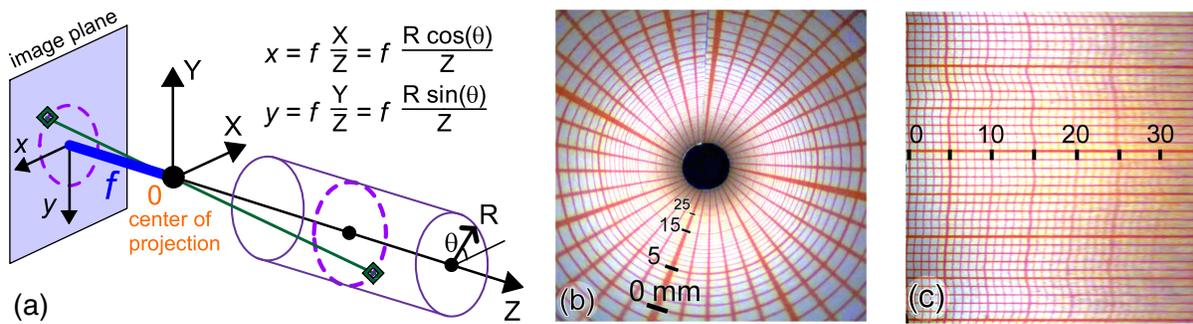
**Fig. 5.** (a) Endoscopic image projection on the CCD sensor of the digital camera; (b) original view of a rolled graph paper; (c) unwrapped view of a rolled graph paper
