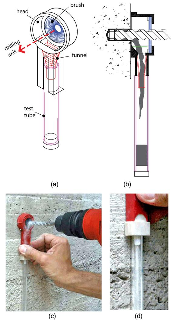
**Fig. 7.** The device for taking sorted samples of drilling powder: (a) sonometric rear view; (b) vertical section; (c) the device in operation; (d) detail of the powder flowing through the funnel (Italian Patent Application MI2009A 001073, patent pending)
