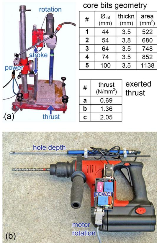
**Fig. 1.** (a) The core drill fitted with sensors for monitoring the operational parameters and variables investigated in the preliminary tests; (b) modified hammer drill for measuring the drilling resistance (as described in Felicetti 2006)
