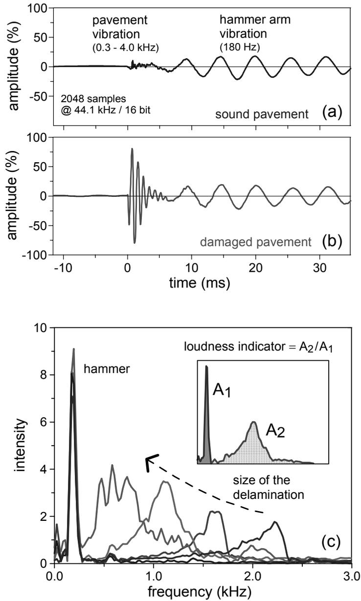
**Figure 4.** Typical recorded signals following a hammer tap on either: a) a sound or b) a damaged pavement; c) frequency spectra at increasing size of the delamination crack and definition of the loudness indicator
