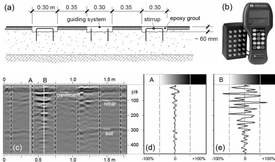
**Figure 8.** a) cross-section of the repaired pavement; b) ultrasonic device for the implementation of the shear pulse-echo technique; c) B-scan across a repaired cross-section and d)-e) A-scans pertaining to a repaired point and to a remaining piece of the old pavement
