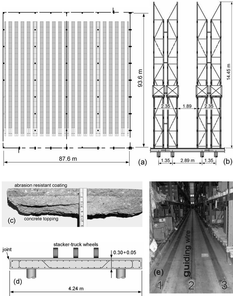
**Figure 2.** a) plan of the investigated warehouse facility; b) cross section of an aisle between the racks; c) concrete layers forming the 50 mm thick pavement; d) ground-slab strip supported by piles and e) view of an aisle and its flooring
