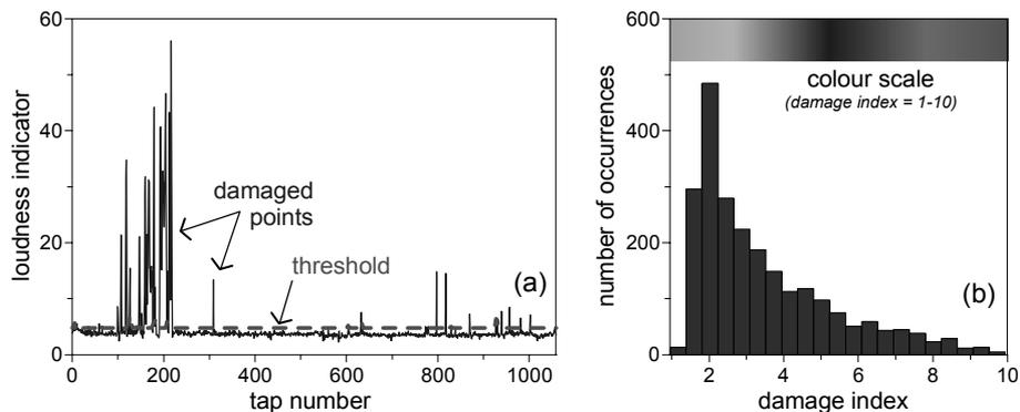
**Figure 5.** a) Loudness indicator along one 80 m line (1 066 taps) compared to the adaptive threshold for distinguishing the damaged points and b) number of occurrences of the different damage levels and associated colour scale for drawing up the damage map
