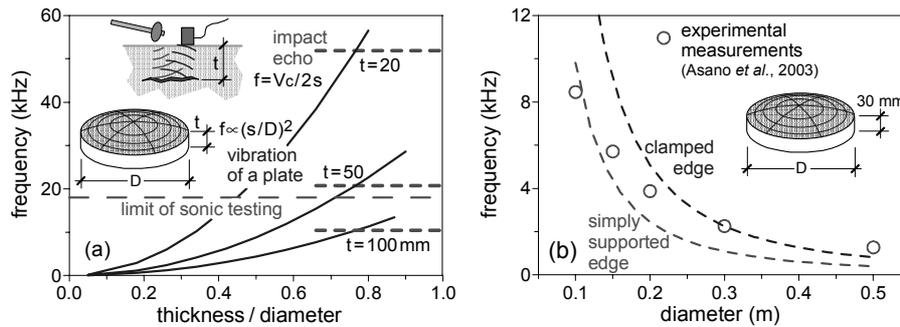
**Figure 1.** a) mechanisms governing the acoustic response of a delaminated layer and b) comparison between the experimental results (Asano *et al.*, 2003) and the natural vibration frequency of circular plates
