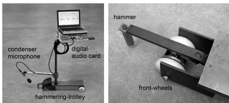
**Figure 3.** The hammering-trolley fitted with the audio acquisition system and details of the hammering mechanism driven by the front wheels
