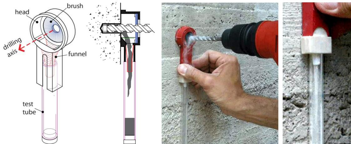
Figure 2. The device for taking sorted samples of drilling-powder: assonometric rear view and vertical section; the device in operation and detail of the powder flowing through the funnel (Felicetti 2009a).
