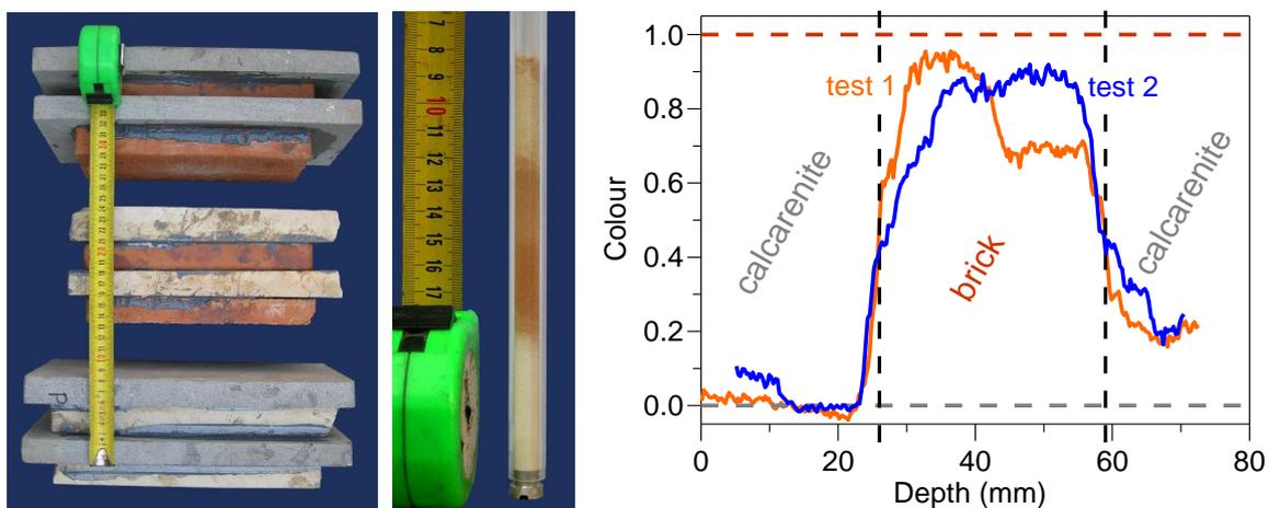
Figure 3. Layered specimens of alternate colours; powder sample extracted from the central calcarenite-brick specimen and diagrams of the colour variations along the powder sample (the abscissa is scaled to the actual depth in the drilled hole).
