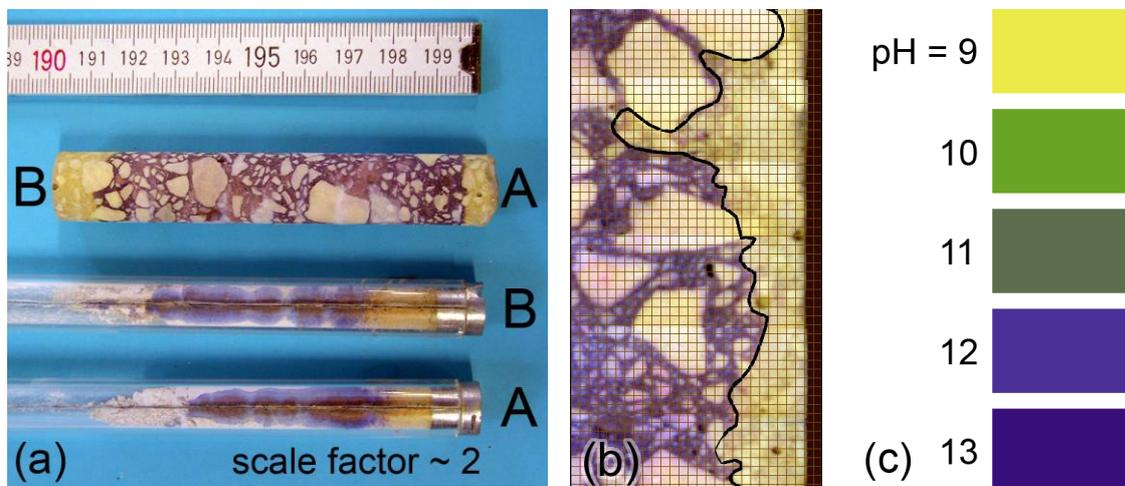
Figure 4 (a) Carbonation depth in a 100 mm concrete cube determined on a micro-core and on two sorted powder samples; (b) local irregularities of the carbonation front and (c) colour scale of the pH indicator.
