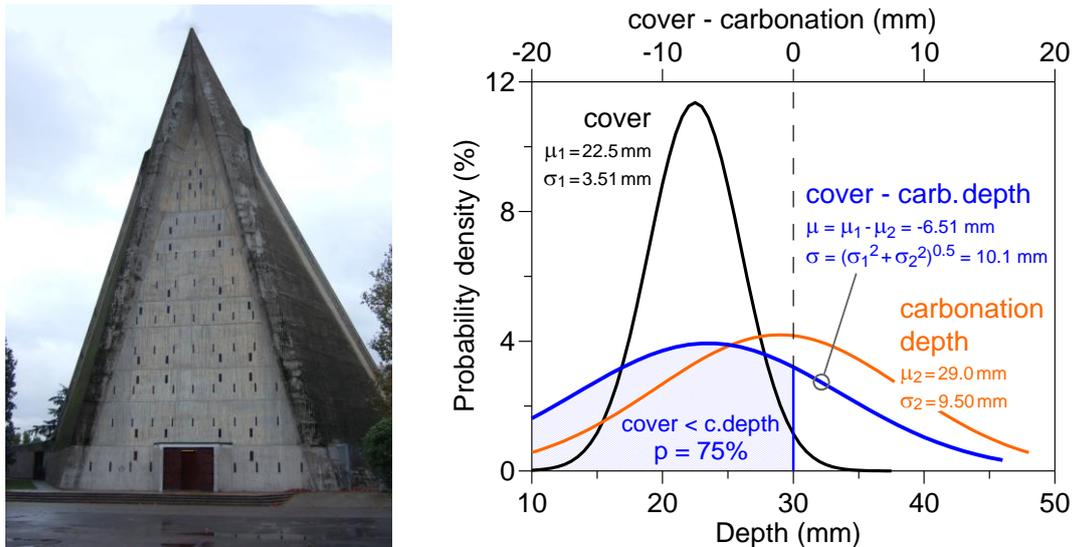
Figure 5. The St. Giovanni Bono church in Milan and comparison among the frequency distributions of the concrete cover, the carbonation depth and their difference.
