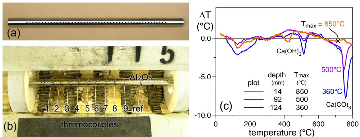
Figure 7. (a) Nickel-chromium perforated pipe to be filled with a sorted sample of drilling-powder and (b) test setup in the split-tube furnace; (c) temperature differentials pertaining to different depths in a heated panel.
