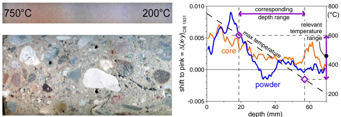
Figure 6 - Discoloration of both a powder sample and a core taken from the same heated panel and corresponding colour variation profiles obtained via the digital image analysis.
