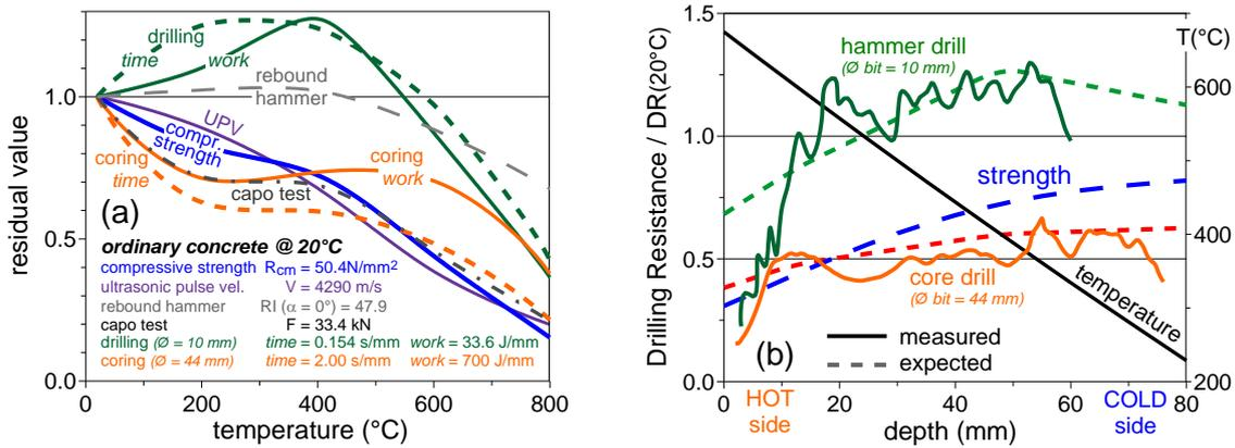
Figure 1. (a) sensitivity to a uniform thermal damage of some common NDTs and of the core- and hammer-drilling techniques and (b) profiles of the drilling resistance indicators in the case of a concrete panel exposed to a steep thermal gradient (675 to 230°C left to right - Felicetti 2009b).
