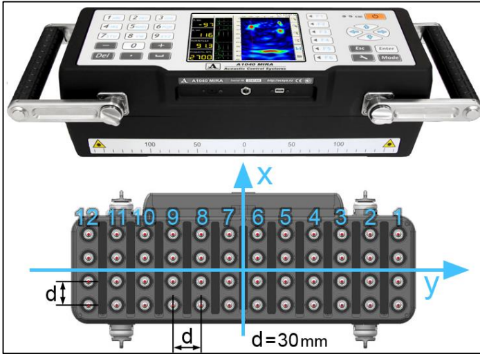
Fig. 1: device and its sensor array
