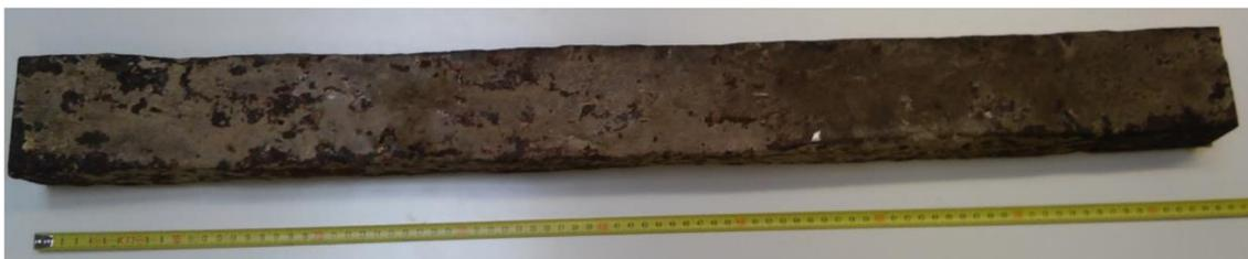
**Figure 1.** Portion of an ancient tie rod from Milan Cathedral (1400 AD).
