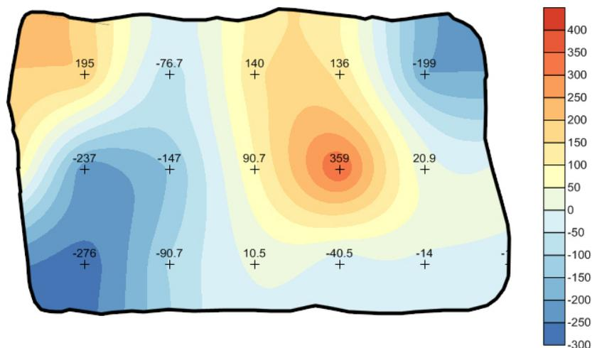
**Figure 3.** Map of the strains derived by ND analysis at ENGIN-X. A non homogeneous distribution of strains is clearly visible.
