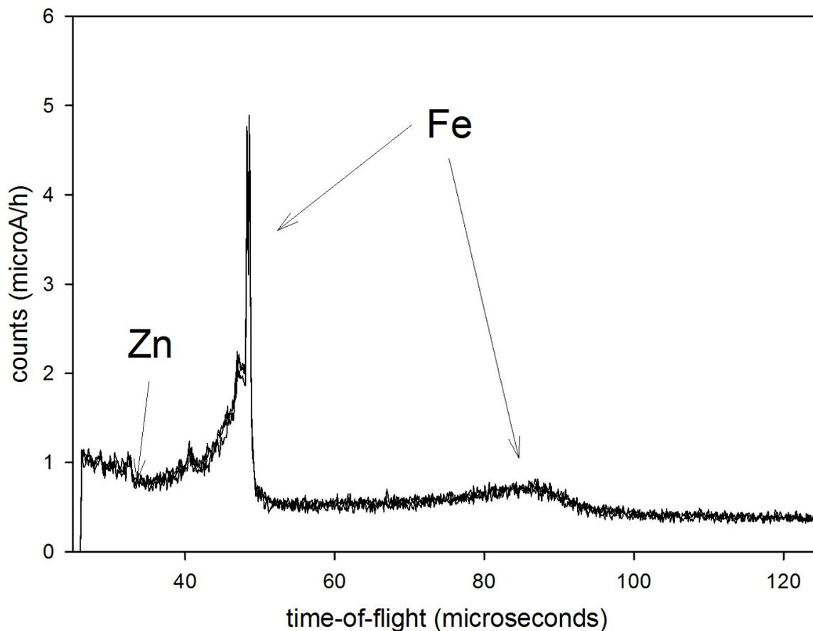
**Figure 2.** NRCA results on iron tie rod. Three different points along a horizontal direction were measured.
