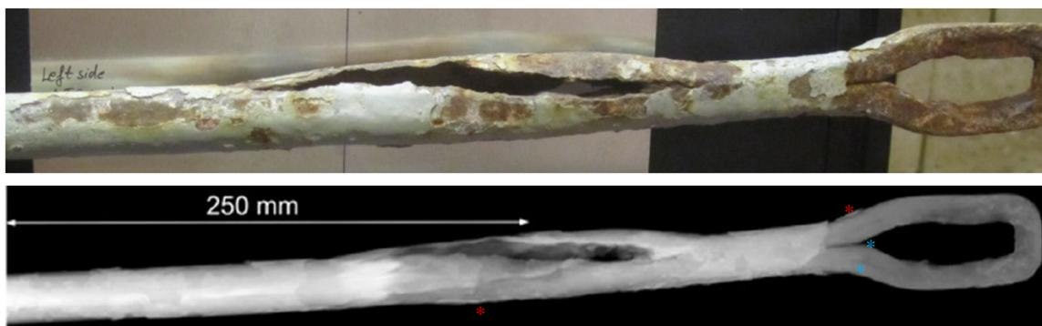
**Figure 5.** Visible appearance and neutron radiograph of another tie rod coming from an external spire. Crackings due to the atmospheric exposure are evident, but also other interesting inner details. See text for further comments.
