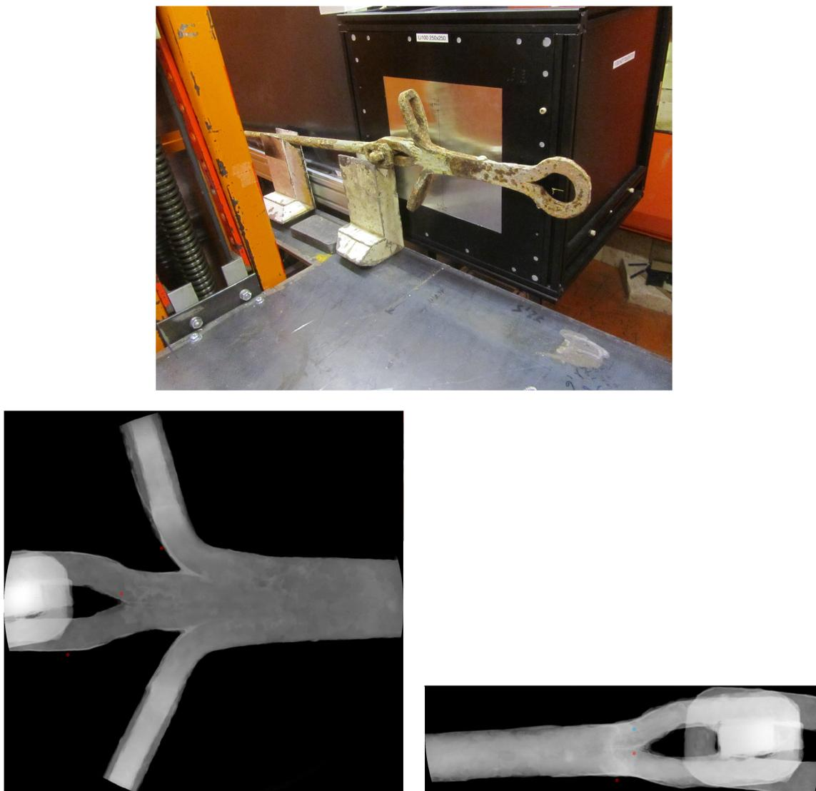
**Figure 4.** Visible appearance and neutron radiograph of a tie rod from an external spire of the Duomo Cathedral. See text for details.
